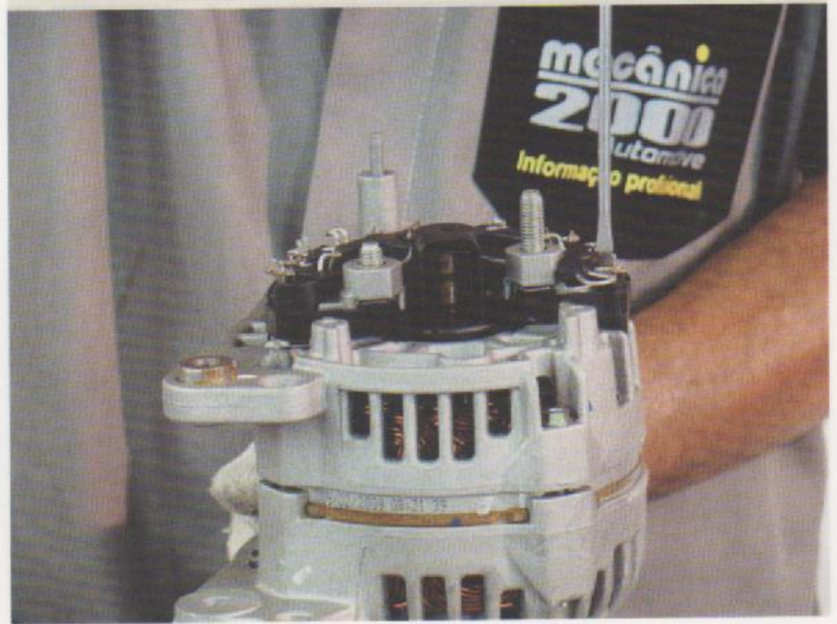
Fig.3 - Descravando as bobinas do estator
